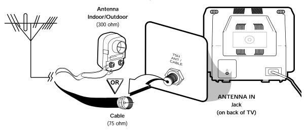
Connect the antenna or cable to the ANT(enna) IN Jack on the back of the VCR.
